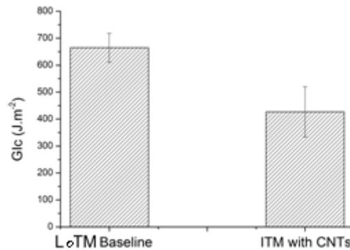
Figure 5: Interlaminar fracture toughness results
