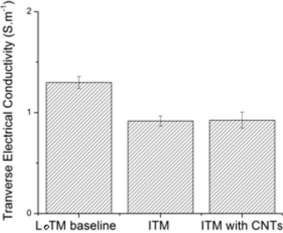
**Figure 4: Transverse Electrical Conductivity of various CFRP materials**
