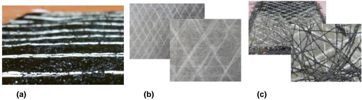
**Figure 3: Forms of material screened; (a) granular masterbatch, (b) melt-blow veil and (c) extruded fibre veil**
