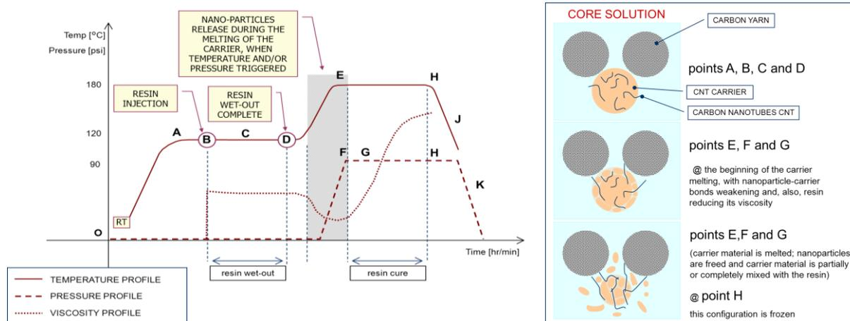
**Figure 1: Typical temperature, pressure and viscosity profile of one LRI process. Figure 2: a graphical representation of expected carrier behaviour during the resin infusion cycle.**
